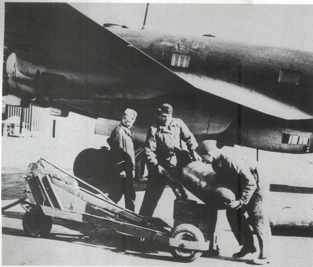
Left: Effort from the whole ground crew was necessary to pull a bomb like a SC 250 onto the modified mounting for cylindrical bomb loads. This picture, taken at Bordeaux in 1942, shows a Fw 200 C-3 belonging to KG 40. The lower rear weapon position normally was fitted with a single MG 15, but in 1942 the position's armament was upgraded by the use of a more powerful MG 131 machine gun.
