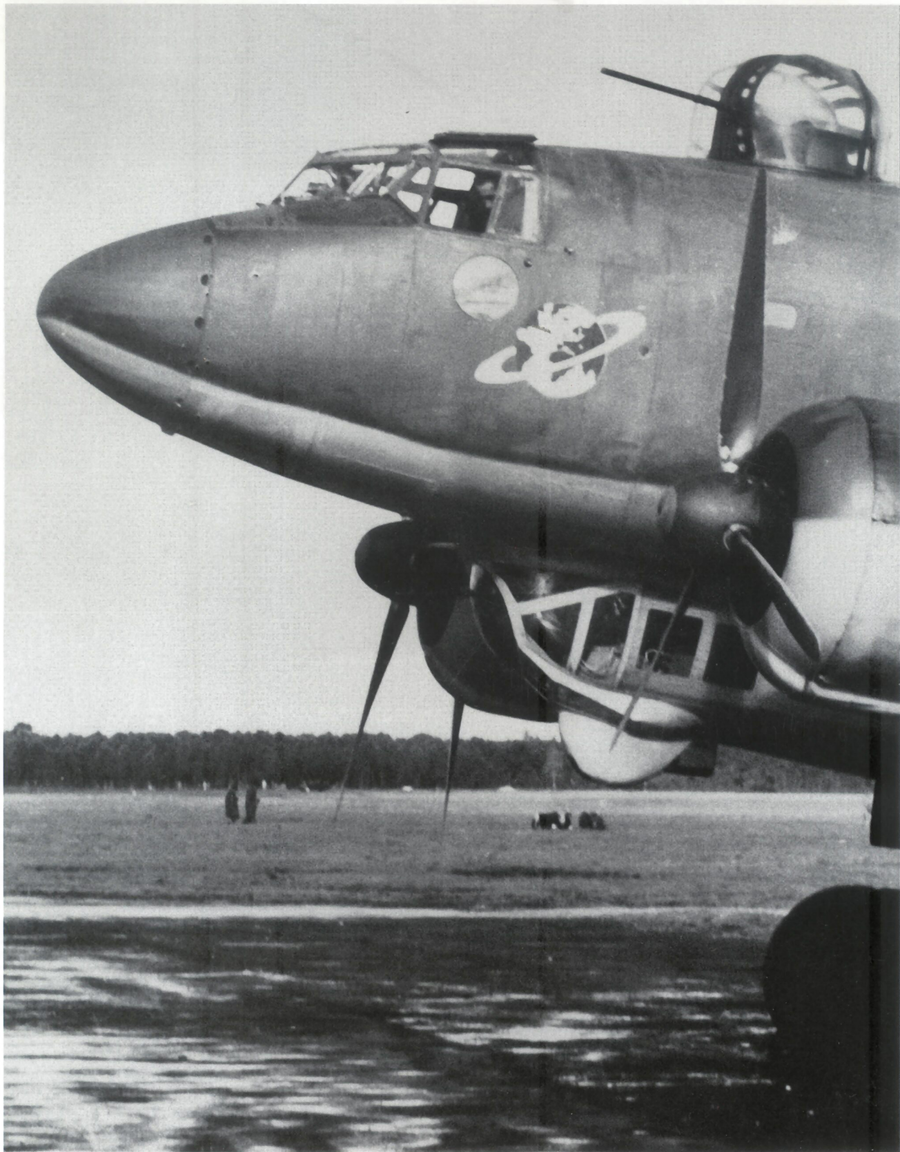
This Fw 200 C-4 is armed with a single MG 151/20 gun on the fuselage roof and a small movable MG 15 fixed in the forward dorsal turret of the aircraft. The large emblem of KG 40 can be seen on the fuselage. Just off the runway, two patrolling German soldiers appear to be protecting both the aircraft and two cows lying on the grass!
